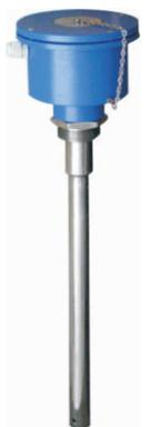
Head mounted electronics converts the capacitance variation to 4-20mA signal for long distance transmission. It is provided with trimpots for SPAN and ZERO adjustments. With no moving parts it is free from wear and tear, rugged and robust in construction. No dead zone like float based instruments.
